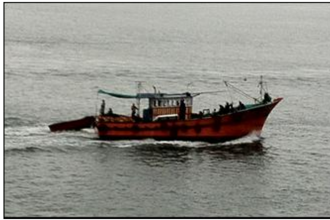
Photograph of ‘chase boat’ towed by a fishing vessel
